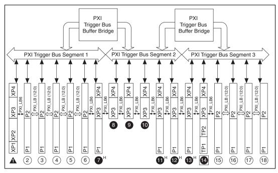
Figure 1-4. PXI Trigger Bus and Local Bus Connectivity Diagram
